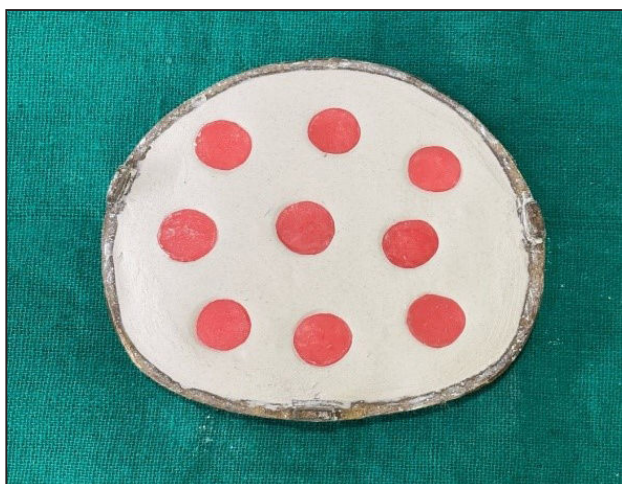
Figure 1: Mold for fabrication of samples
