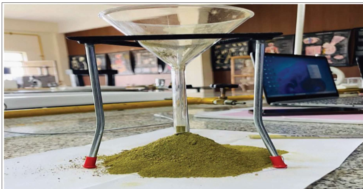
Fig. 4: Angle of repose
