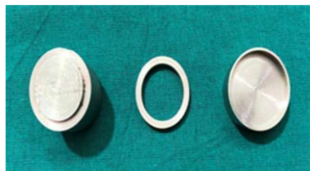
Fig. 1: Stainless steel Die (1.5 mm x 50 mm)
