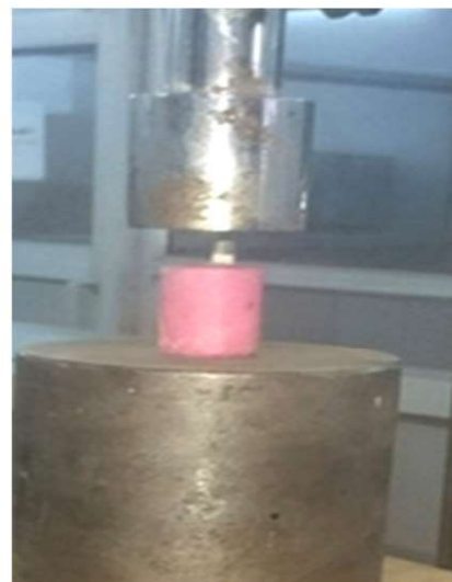
Fig. 7: Pull- off test on UTM
