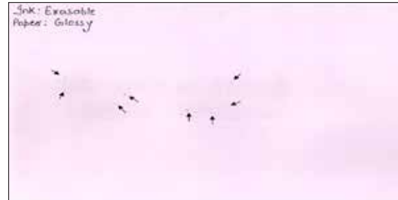
Figure 5: Few traces at the end of strokes reappeared when writings on the glossy paper is removed by using friction (rubber erasure)
