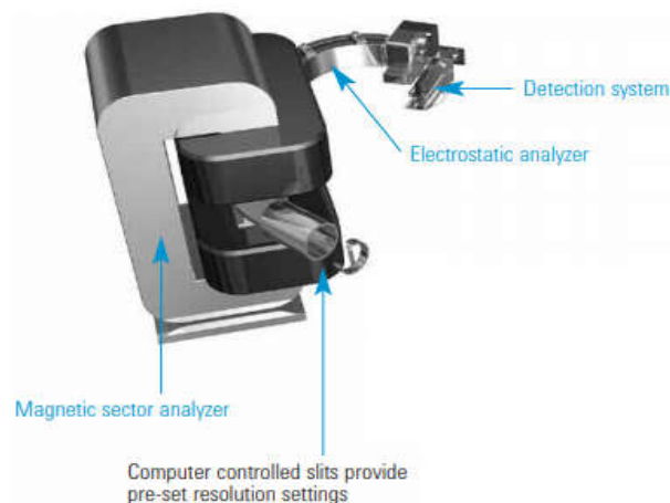
Fig. 9: Schematic of Magnetic Sector Analyzer.
